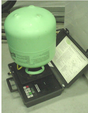
Charging Cylinder on Scale
